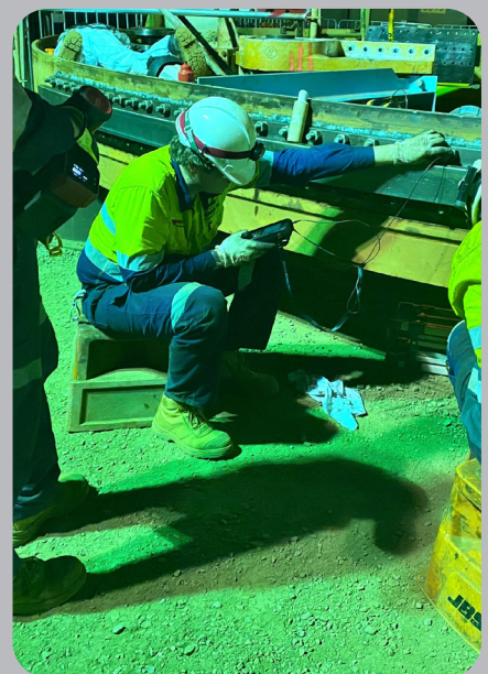
Tension analysis with Ultrasonics
